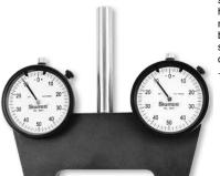
Offers accuracy, convenience and significant time saving with the common shop task of tramming the head of a vertical milling machine. This must be done regularly to ensure squareness and perpendicularity between the spindle and work surface. The spindle square is easier to use and more precise than the traditional method of tramming with a dial test indicator. .001" Grad, 0-50-0 Dial; .250" Range.
